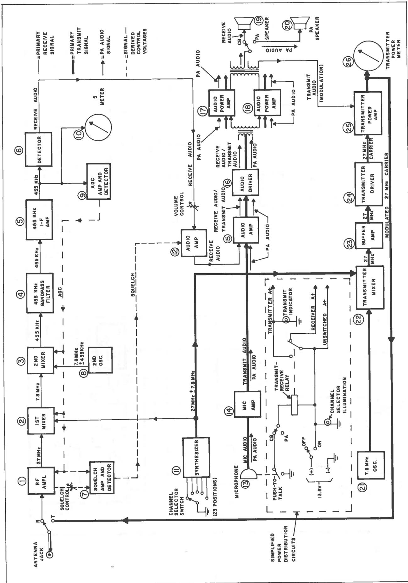
Fig. 22. Block Diagram of Typical AM CB Transceiver
