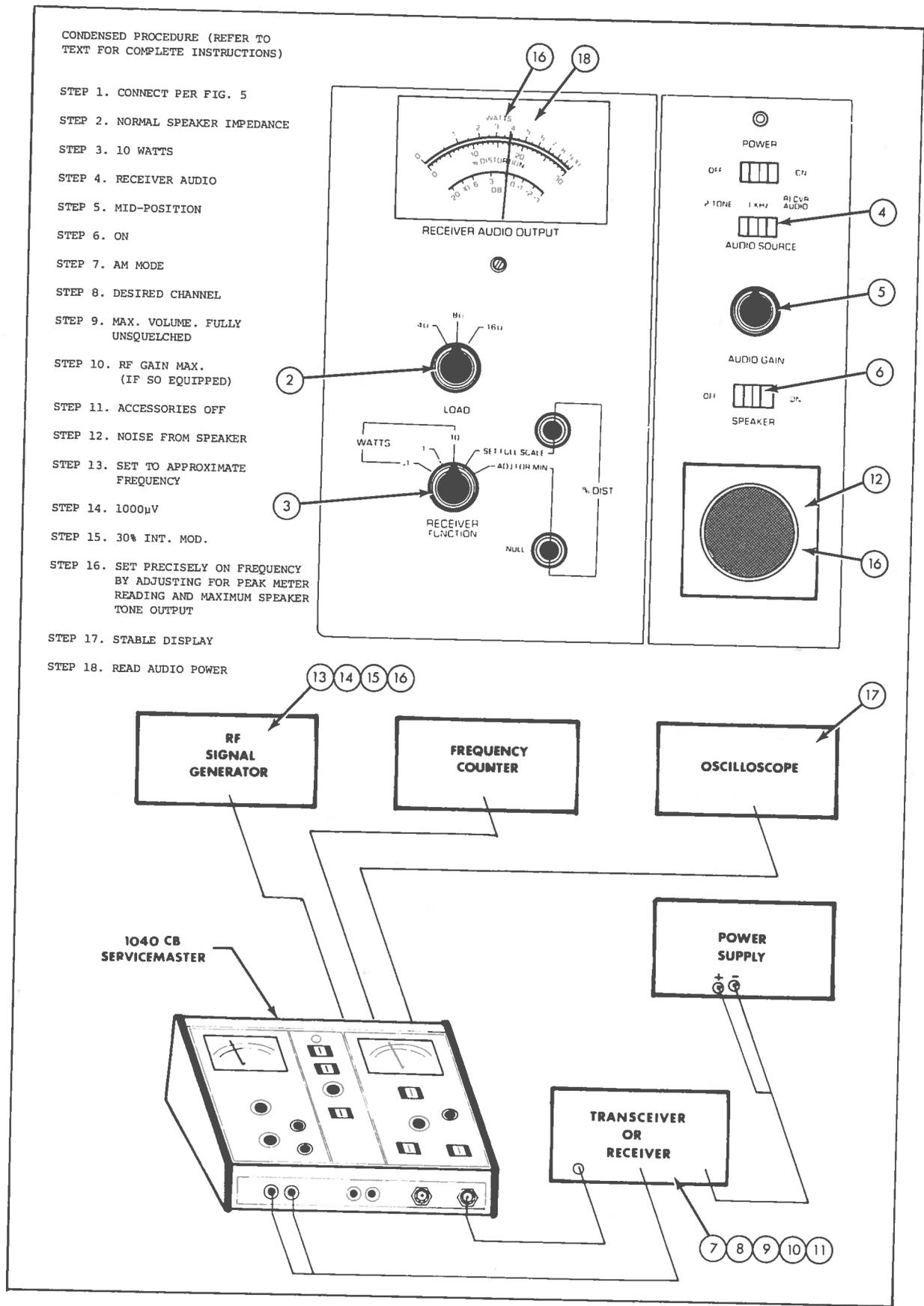
Fig. 9. Receiver Audio Power Check
