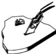
FIGURE 7. HOW TO CONNECT A WIRE TO A TERMINAL
